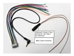
Some radios will have a 3.5mm port located on the back of the radio. For radios with this option, plug the male 3.5mm jack directly into the back of the radio.
