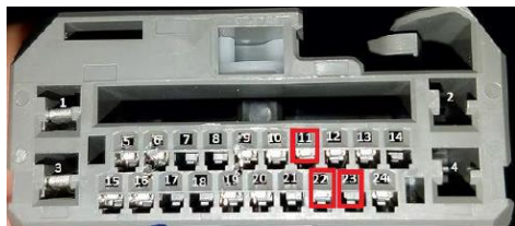
This is the pin view of the radio connector in the vehicle
