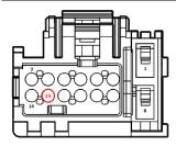
This is the pin view of the 14 pin radio connector in the vehicle
