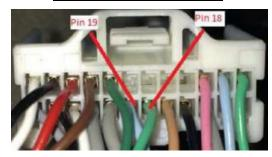
This is the view of the 24 pin radio harness in the vehicle.
