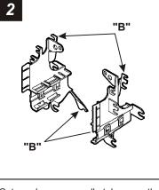
Cut and remove all tabs on the Mounting Brackets EXCEPT tabs "B". (The tabs can be identified by the stamped letter by each tab). Skip to the Installation Instructions for ALL VEHICLES on Page #3.
