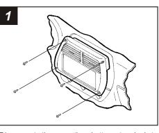
Disconnect the negative battery terminal to prevent an accidental short circuit. Remove (4) 3/16" Allen Screws from the radio trim bezel and remove the bezel. Remove (4) 10mm bolts securing the factory head unit and disconnect the wiring.
