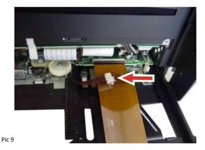
**STEP 10:** Carefully fold and insert the flex ribbon cable inside the navigation unit cavity.
