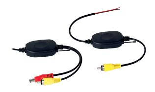
The iBEAM TE-TXRX transmitter and receiver is designed to save time by not having to run a video cable through a vehicle. The transmitter has a video and power plug that connects with our iBEAM cameras to make installation a breeze. The receiver has a standard composite video cable that will plug into most video screens.
